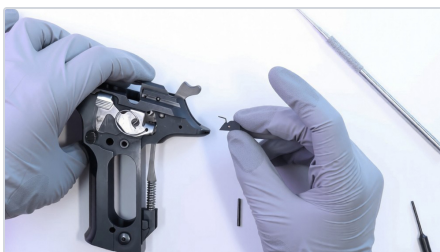
Step 1 — hammer stop and spring positioned in the frame.
