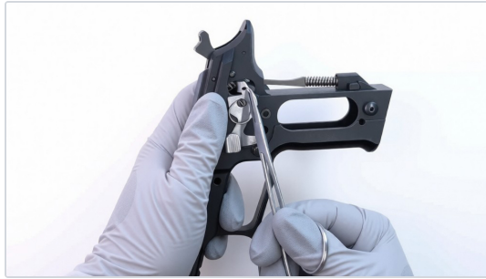
Step 3 — the Forceps set the spring while the magnet still holds.
