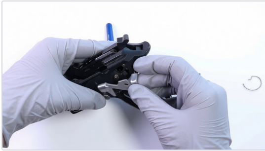
Step 2 — lever and spring positioned against the held bearing.
