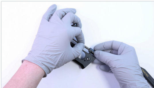
Step 2 — mainspring and seat slid onto the hammer strut.
