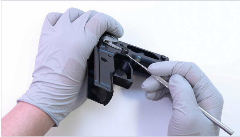
Step 1 — the Needle Tool depresses the mag catch stop as the catch is pushed in.
