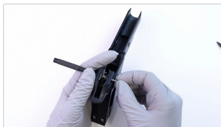
Step 4 — the sear pin follows the punch out.
