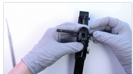
Step 4 — the hammer stop pin drives the punch out.
