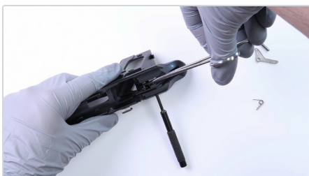
Step 3 — sear, sear spring and safety lever placed with the Forceps.
