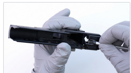
Step 5 — tensioning the sear spring.
