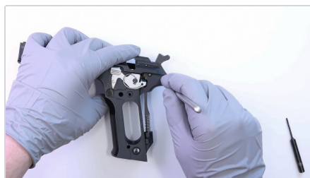
Step 2 — the Needle Tool brings the bores into alignment.
