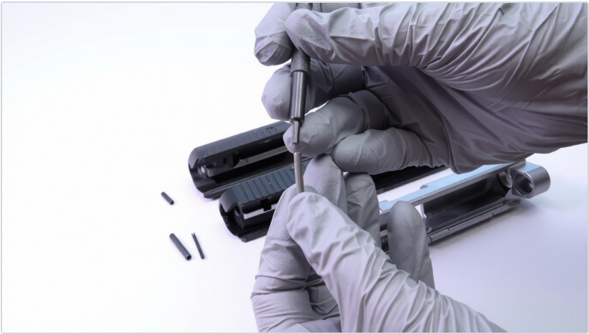
Match the punch face to the pin type before driving.
