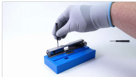
Step 3 — drive the pin with the punch square to the bore.
