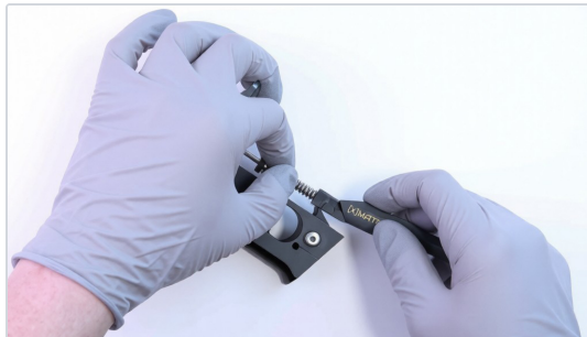
Step 3 — the Seat Tool engaged squarely in the seat.
